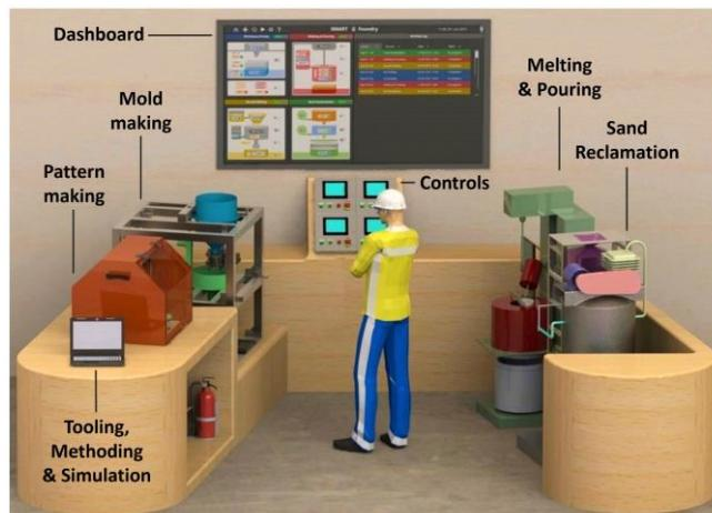
Fig. 11. SMART Foundry units, layout and dashboard
