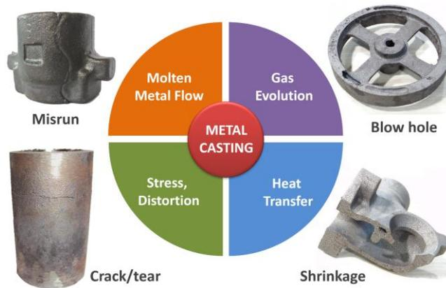
Fig. 2. Major casting defects related to process phenomena
